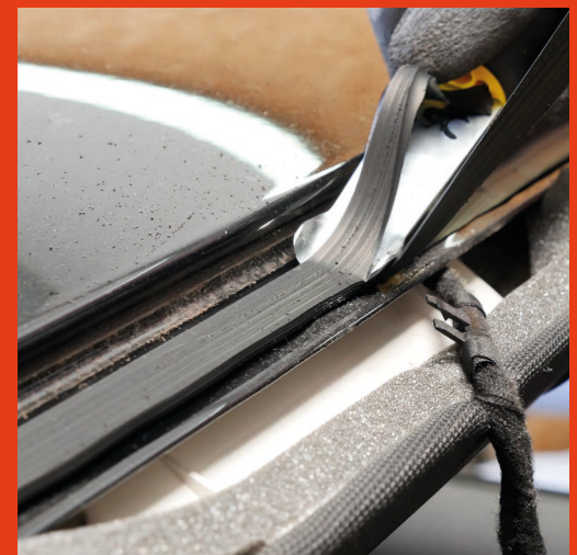
The correct adhesive thickness is retained so that subsequent re-gluing is possible without any problems.
