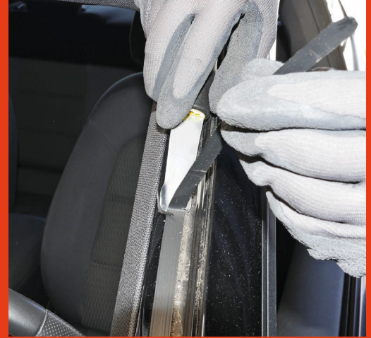
The blades have a curved back to remove the PU adhesive.
